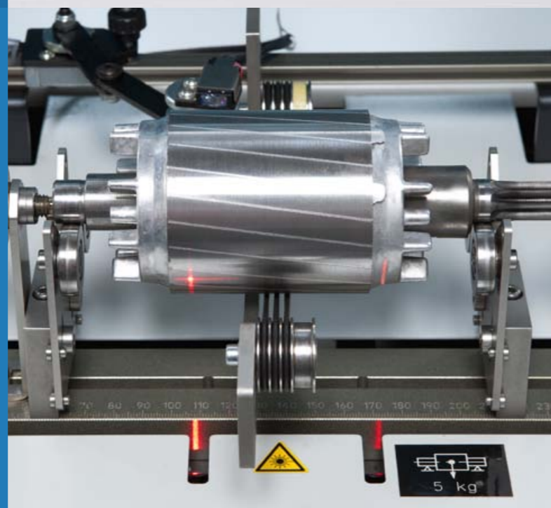
The line laser ensures the clear display of the measurement planes (Pasio 5)
