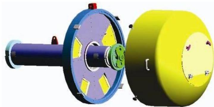
Devices with spindle bearings and a chuck, like the one shown here for an LPC booster subassembly, enable components to be balanced in which the adapter surfaces that determine the rotational axis cannot be supported directly on the balancing machine. As tools for a measurement operation, these devices also fulfill the function of measuring equipment<sup>1</sup>.
