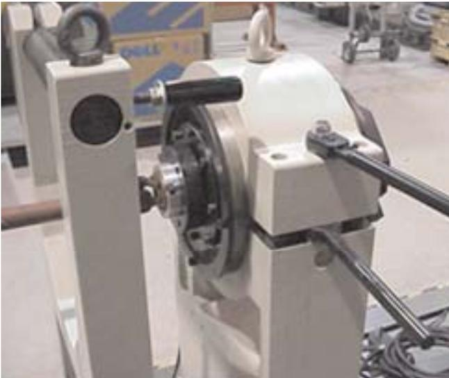
**Figure 4. HK40 balancing machine support and safety pedestal.**
