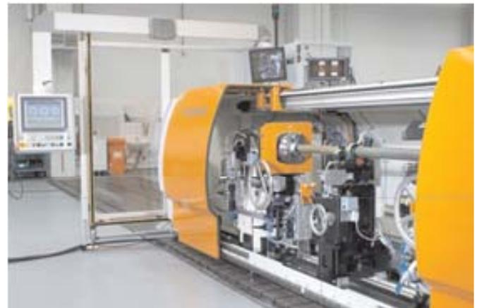
**Figure 3: Schenck 200X Driveline Balancer**
