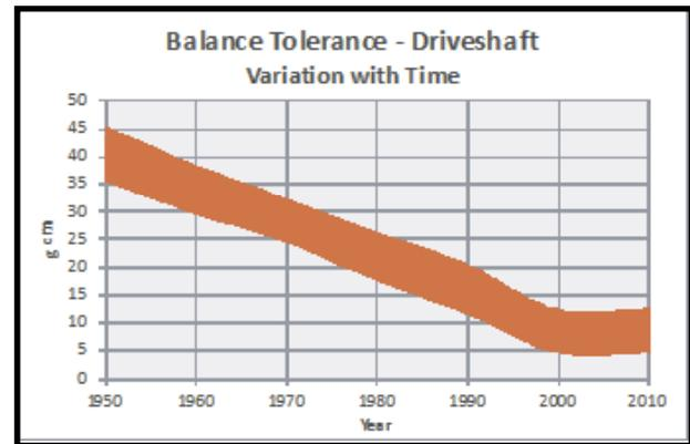
**Figure 2: The vanishing driveshaft tolerances**
