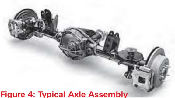
**Figure 4: Typical Axle Assembly**
