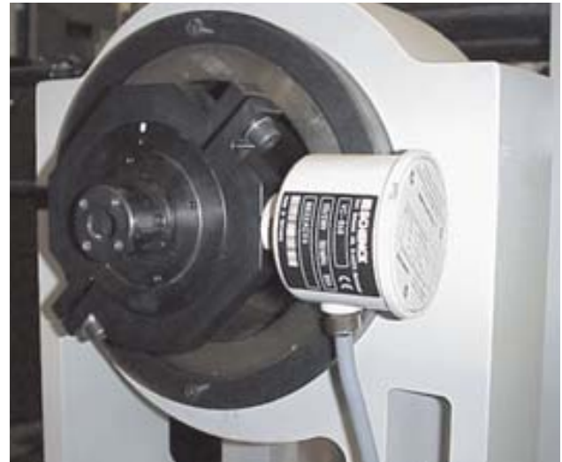
Figure 5. Our Force Monitoring System is designed to shut down the HK40 balancing machine should excessive vibration resulting from a resonance condition be sensed.
