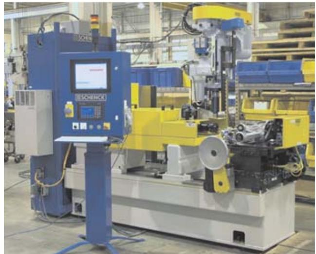
**Figure 6 Standard Horizontal Axle Balancer (Without Guards)**
