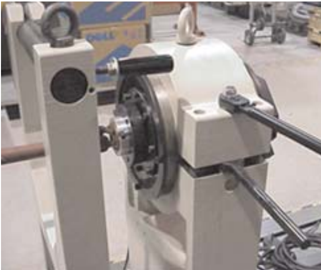
Figure 4. HK40 balancing machine support and safety pedestal.
