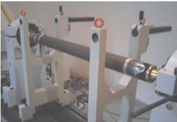
Figure 1: Fixed Spindle Pedestals and Safety Pedestals with Tooling and Driveshaft
