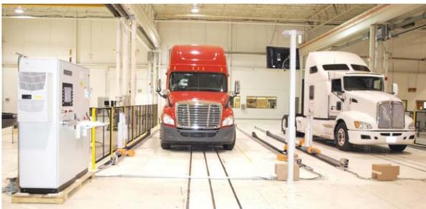
Due to the newly developed chassis geometry test stand for trucks, we are able to deliver a cost-effective measuring test stand. Even the measurement of steering inclination at the front axle and a steered rear axle is possible.
