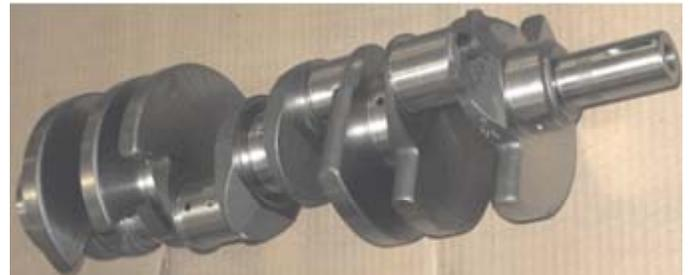
Figure3: Typical Crankshaft
