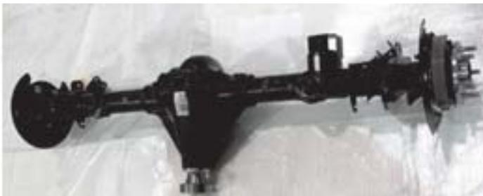
Figure 1: Complete Balanced Axle Assembly
