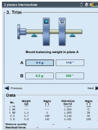
**Phase measurement** gives the user an advanced set of tools to distinguish machine faults. For example - it can be used to determine the unbalance type - static or dynamic, alignment errors, bent shaft detection, and/or loose foundation...This is a synchronous phase measurement, which means that the amplitude and the phase angle of the vibration sensor are calculated with respect to the laser pick-up.
