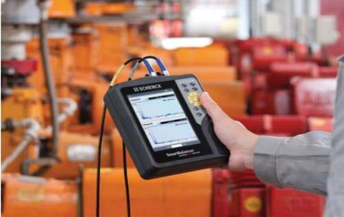
Probably the most common problem is unbalance. Unbalance (an uneven distribution of mass around the axis of rotation) can result when individual components have not been properly balanced prior to assembly, errors in the assembly of these components, or operation conditions.
