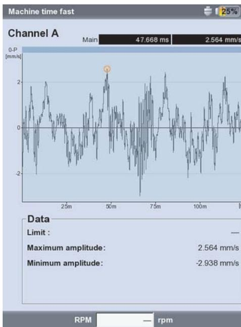
This makes it useful in the identification of transient, short duration form unstable and irregular vibrations caused by such things as mechanical looseness, transient impacts, etc. – they can negatively affect the outcome of a field balancing job. Oscilloscope functions are also useful for identifying sensor problems.
