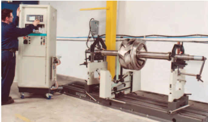
Hard-bearing balancing machine saves time by eliminating the need for numerous calibration runs
