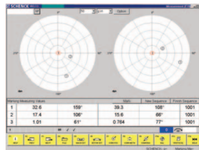
A mass recalculation program provides an effective visual to fine tune the correction process.
